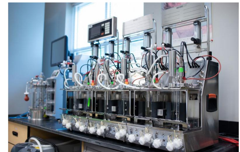
Electrochemical monitoring is being developed for use in bioreactors at various scales. Future applications of this technology include monitoring biopharmaceutical processes in conjunction with studies in Dr Sarah Harcum's Cell Culture and Fermentation Optimization Laboratory at Clemson University.
